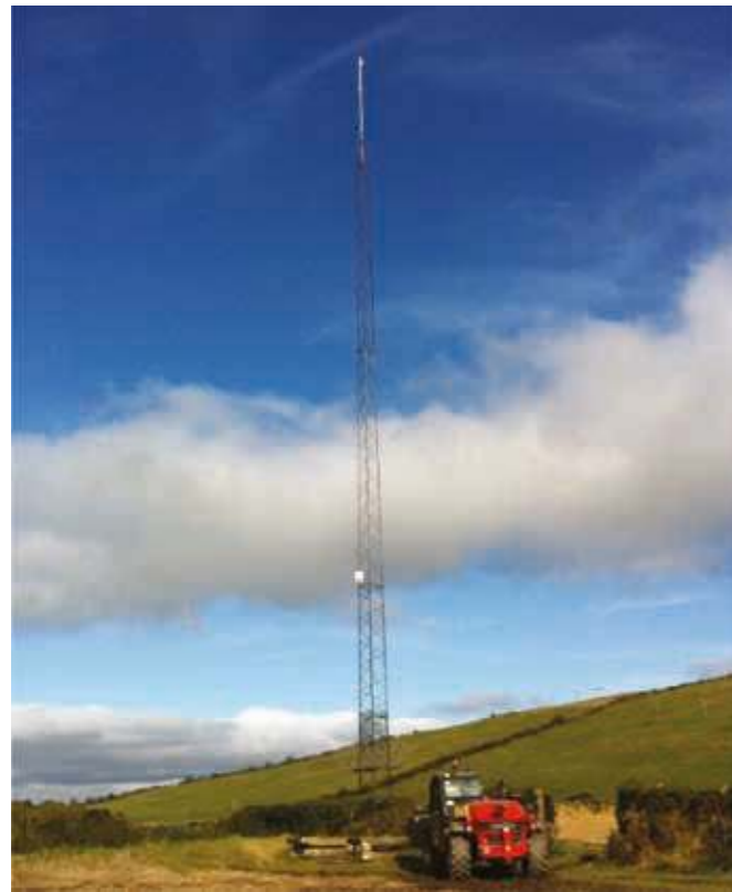
Figure 26: A Typical Wind Mast Set Up (image courtesy of Element Consultants Ltd)
