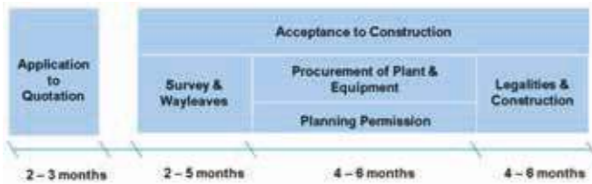
Figure 39: Grid Connection Timescale (Planning Required) (image courtesy of NIE)
